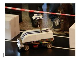
The circular track represents a winding country road. The cars must drive three rounds within a possibly short time. In the third discipline "Circular track with obstacles", parking cars are distributed on the own lane as well as on the left lane such that evasion requires the use of indicators. Of course, the car may not strike the obstacles.
