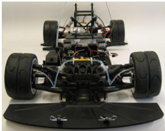
For its later use at the chair, the experimental vehicle shall be equipped with various, distributed and networked electronical control systems. It must be possible to carry out different driver-assistance-systems with various configurations. The experimental vehicle has to be conceived in a way that future enhancements with control elements, sensors or actuators are possible.
