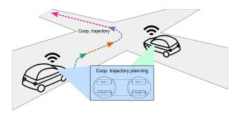
There exist two major challenges in distributed trajectory planning. Firstly, planned trajectories need to be collision free. Secondly, the planning algorithm on board of the vehicles should be real-time compliant. This is challenging due to the complexity of the trajectory planning problem, which grows exponentially with every road user that is taken into account.
