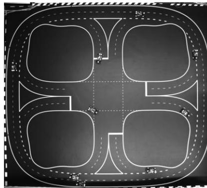
FIGURE 1 ROAD NETWORK IN THE CPM LAB WITH MODEL-SCALE VEHICLES.
